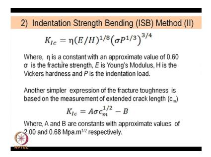
And therefore, one can have once again an expression indentation strength bending by this method K i c is this expression. So, where eta is a constant with an approximate value of 0.6, sigma is the fracture strength, E is the young's modulus, H is the Vickers hardness and P is the indentation load, which we have, which we have been added, which have been used or applied.
