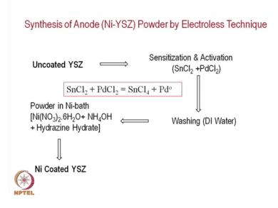
Normally one users nickel and YSZ just mixed together which may or may not be the right kind of connectivity here at a particular technique has been used which is called the synthesis of anode powder by electro less technique. Let me try to describe this process this very simple process where the YSZ powder is being quoted each of the individual YSZ powders been coated with nickel or metallic nickel right so that you get every YSZ is coated with nickel and whenever such nickel coated.
