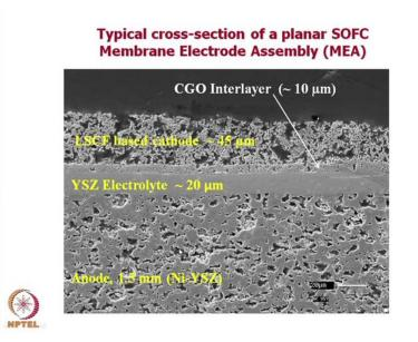
So, this as shown you earlier, this is the typical microstructure of the cross section as we have discussed earlier that the anode as well as the cathode is a porous structure in between you have a dense electrolyte, YSZ electrolyte. In this particular case, it is about 20 micron thick in addition 4 th layer here which is called the cathode functional layer. In this case is about 10 micron thick and it is a basically a gadolinium doped cerium CGO interlayer.
