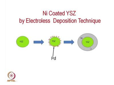
Yes, this is kind of a pictorial representation of what actually happens this is bayer powders. YSZ powders than you put a the palladium sensitization. So, far palladium particles actually gets adhere to the surface of an YSZ and then after the electro less solution it makes a is put the electro less solution the nickel a good coating of the nickel oxide and nickel metallic nickel. Now, this is not nickel oxide this is metallic nickel produced over YSZ.
