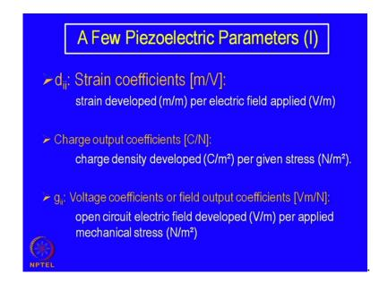
Well, we will just have a brief discussion on this. We will discuss them in details later on, but to start with we will introduce actually 4 different coefficient. One is the strain co efficient because the 2 parameters are interconnected; one is the electric field and the mechanical strain.
