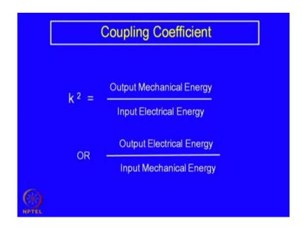
And, so the coupling coefficient basically is the ratio of the 2 energies and therefore, a number.
