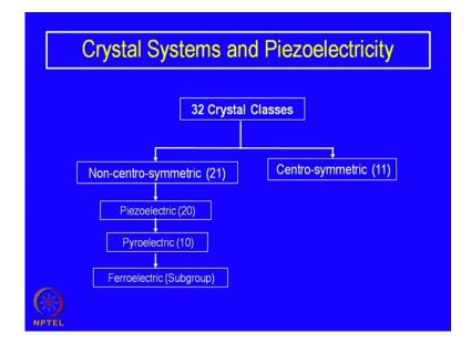
Well, this can be summarized in this form of a flow diagram; 32 crystal classes has been sub divided into 2 groups. One is non- centro-symmetric 21 of them and another group is centro-symmetric so 11. So, these 11 do not have piezoelectric property. Now, out of 21; 20 have a piezoelectric property as already mention for someone that is consideration it does not show piezoelectricity.
