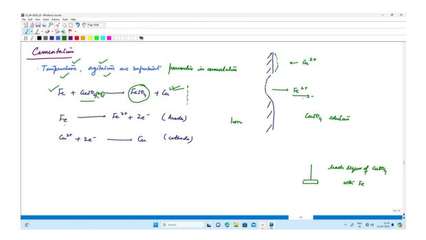
But essentially, we are also losing iron from the iron disk itself and the iron is getting collected into the leached liquor solution. There are multiple other methods by which we can recover valuable products from leach leakers. For instance, we can think of precipitation or crystallization.
