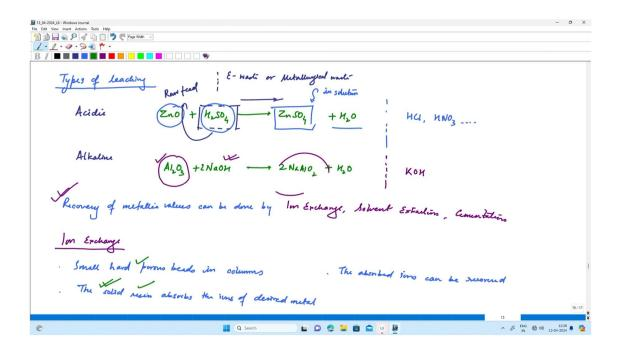
The desired metal is absorbed on the solid resins and since it is absorbed on the solid resins, it can be recovered back. The ion exchange on the solid porous beads is possible, which is why this process is called ion exchange. Size and valency of ions are of immense importance. While we think of ion exchange, concentration of ions in the solution, it should have some minimum quantity of ions in the solution that we are trying to extract.
