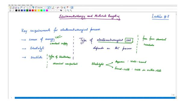
The type of electrolyte that we are using either it is fused salt electrolysis or aqueous electrolysis and of course the type of electrodes that are being used the chemical composition, anodes and cathodes and based on all of this and supporting the most important, the electrometallurgical cell that encompasses the electrometallurgical process. We now move towards the classification. This is basically classification of electrometallurgical processes.
