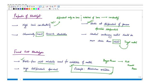
There are some key disadvantages of fused salt electrolysis. Of course, it is one of the most important methods by which we can extract metals so, if we have a molten bath that contains our metallic ions, we should be able to extract the metal under the required temperature, composition and electrical energy. The constraints that we supply, we should be able to extract the metal, but there are some disadvantages.
