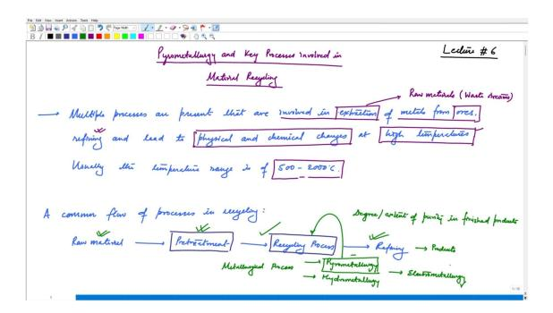
Pyrometallurgy is one of the possible routes of recycling used for metal recovery, refining and thermal treatment. Not just for extracting metals or refining, we can just simply think of thermal treatment which could lead to changes in phases, changes in properties this could be physical properties or chemical properties and based on these we can think of developing further processes. Now, let us begin by thinking of calcination.
