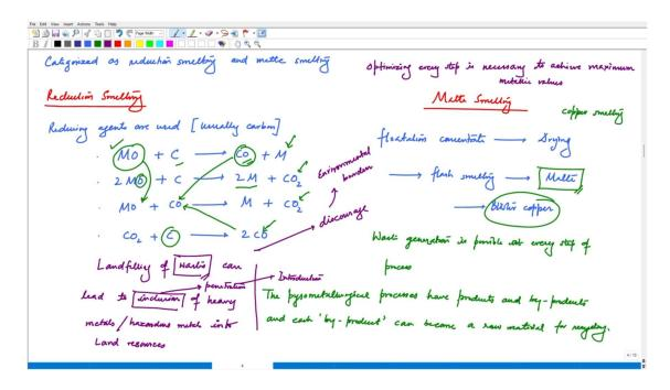
Again, we begin with this raw material and we have CO. We have this and this. This could also lead to the formation of metal, but this time we are getting CO<sub>2</sub> and the CO<sub>2</sub> in a given system could be used by carbon itself to give us 2CO and this 2CO could be used for the previous reaction.
