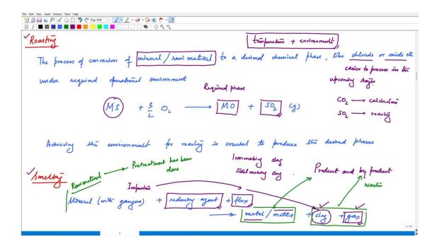
This could be reduction smelting and matte smelting and we have already seen that the common reducing agent could be carbon. Suppose that we begin with metal oxide, reacts with carbon, CO is formed and we get metal. Similarly,
