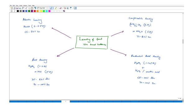
Then we can have let us say 65 to 100 % manganese and 70 to 100 % zinc recovery and these are some valuable routes by which we can produce some valuable materials from battery masses just by flipping our method of leaching. In this class we have covered a wide variety of processes for zinc-based batteries. In the upcoming classes we will be focusing on lithium-ion batteries and its recycling. Thank you.
