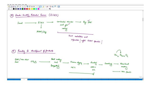
One has to add  $Fe_2O_3$  to zinc dust and then you can make these types of products. The other important alternatives for using zinc dust are basically hydrometallurgical let us say leaching. Leaching with iron powder addition and, iron powder is used as an additive here it is not used of course, it is not used as a reagent. One should really mind what we are adding when and what is its purpose. We can have zinc dust and, zinc dust is coming from various sources not just steel making.
