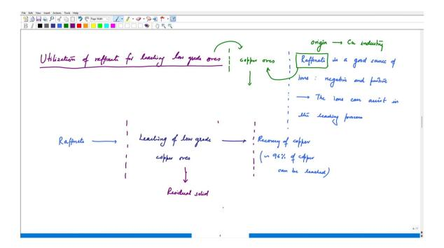
Just by using a waste solution that contains the ions, it is possible to extract a really good amount of metallic content from low grade ores. Low grade ores which are normally used by hydrometallurgical processes. What happens it is just a common way of understanding that the higher concentration of metallic values, the ores that have these types of metallic values are normally subjected to pyrometallurgical route.
