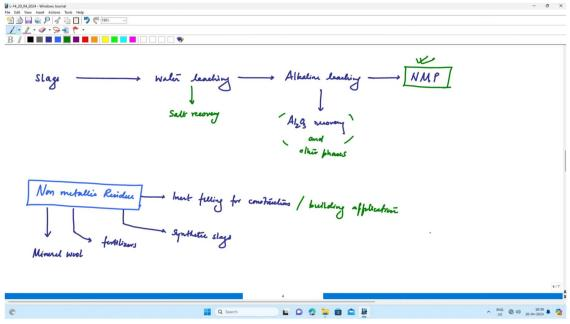
We see that we have multiple methods of recycling the salt cakes. We'll now discuss the last method of recycling the salt cakes, the aluminium slags. There again the first step that we look at is basically water leaching wherein we are interested in basically salt recovery from solution. But at the same time what we are actually making is cement clinker and for that we would be using the residual solid. And to make the cement mixture we would be also needing the addition of other raw materials.
