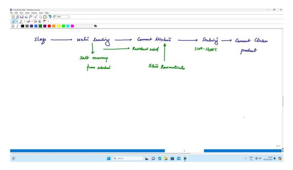
What we see here is the utilization of slag, utilization of salt cakes such that all of the phases are extensively used. Of course, the utilization of each and every phase may not be possible but at the same time the utilization can be done extensively. We've already seen if comminution can help us in recovering metallic values if at all it is present we should be doing that.
