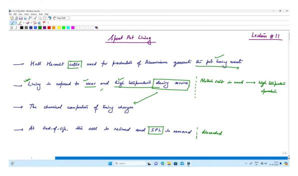
We will first begin by understanding the chemical composition of the spent pot lining. We have just seen that for a lining we must have some refractory bricks and it has to be covered with the carbon lining that was the initial composition but after service we get a very different set of phases attached to the spent pot lining. Normally, we get two cuts, two cuts of SPL.
