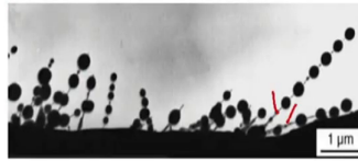
Figure 5.32 Carbon nanotubes produced in an electric arc. During this process, the arc causes the graphite to melt. The outside of the droplets cools at a faster rate, leading to the formation of glassy particles. The liquid carbon inside the drops cools so slowly that it becomes supercooled and later crystallizes as nanotubes, dragging out some liquid carbon as droplets (http://www.gatech.edu/news-room/release.php?id=516). (Reproduced with permission by Walt de Heer.)
