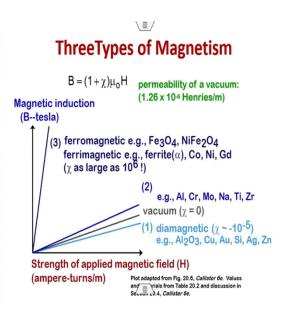
That is what we said the three types of magnetism. You can have a high response that is ferromagnetic material like  $Fe_2O_3$  ok, hematite, magnetite basically not hematite, magnetite or nickel ferrite, Fe, Ni,  $Fe_2O_3$  F<sub>4</sub> ok. They are ferromagnetic. You can have ferrites like alpha iron, cobalt, nickel or gadolinium where this chi value is very high ok.
