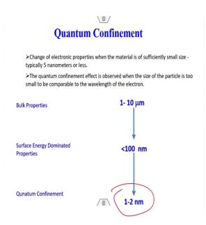
First of all the first one is more important than the second one. First of all, quantum confinement effects are nothing but change of electronic properties when the material is sufficiently small size. Typically 5 nanometer or less and this effect is observed when the size of the nanoparticle is too small to be comparable with the electrons wavelengths of the electrons.
