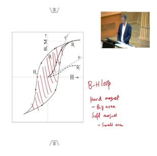
But this is the complete picture of B-H curve ok forget about these things what I am showing here. So, as you can clearly see it increases increases, increases reaches saturation value then you decrease this B-R correspond to remnant magnetism. And then you go to negative value of H for which the B goes to 0 that is known as the coercivity right, this is the coercivity.
