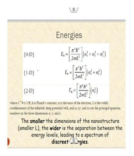
And this can be extended to further 2 D, 3 D ok depending on the size of system. Depending on the type of system as I said its basically 3 dimensional nano particle have a 3 dimensional electronic confinement, 2 dimensional nano particles have a 2 D electronic confinements, sorry 1 electronic confinement and 1 dimensional nanoparticles will have 2 D electronic confinement ok.
