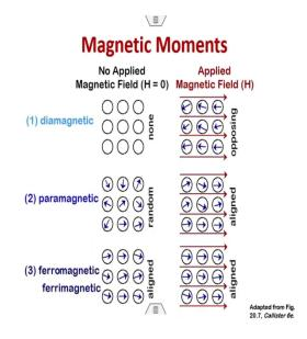
Now, what actually happens atomistically. Your diamagnetic material you have no magnetic field nothing happens. There is no magnetic moment basically present in the atoms or molecules. The moment you applied, magnetic field, magnetic moments will built in very weak magnetic moments will built in, but then they will oppose the applied magnetic field.
