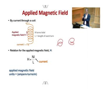
Now, what is the effect of applied magnetic field right. This is the electronic sub structure and all these steps. As you know if I have pass to a pass a current to a coil, we can generate a magnetic field ok. It depends on a number of turns and the length of each turn right. So, the relationship between applied magnetic field and the current is given by this its NI/L, why NI, N is the number of turns, I is the current and L is the length of each turn ok.
