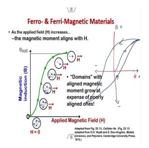
So, let us now focus on ferro and ferrimagnetic materials more. So, it is very clear if you apply magnetic, field there is a huge huge change in the interaction between the spins in the present in the ferromagnetic material and the applied magnetic field and this will lead to magnetization ok. Or this magnetization is measured in terms of magnetic induction ok.
