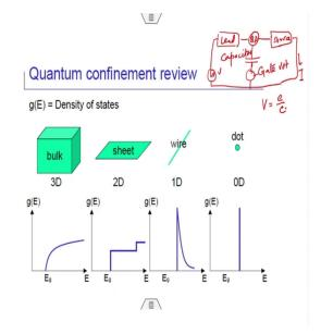
How does it look like? That is what it looks like. If you plot density of states g(E) here versus energy for a 3 D or a bulk nanomaterials, well all the dimensions are more than N nanometers then its looks like this it is a continuous energy band spectrum basically the moment it become a sheet like 2D ok.
