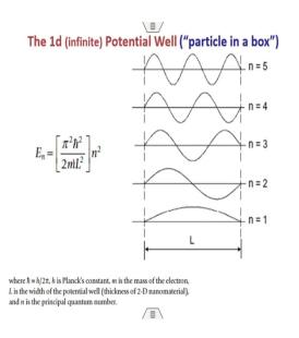
Well, that is this case in a potential well, if a potential well of length 1 depending the values of n you can have different you know allowable energy levels, like n equal to 1 2 3 4 5 right that is what is important.
