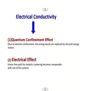
There are two important aspects of electrical conductivity. One is the quantum confinement effects I taught you and this is mainly because of the electronic energy confinement, electronic state confinement and that means, the energy bands will be replaced by the discrete energy states in the nanoscale. That is something which is important in all properties almost like electrical, magnetic, thermal, optical and also acoustic properties of nanomaterials.
