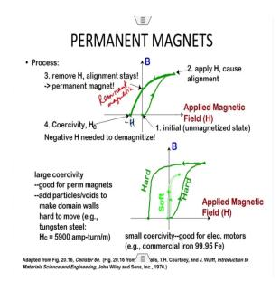
So, if you this is what this is the initial magnetization state and then it causes alignments completely then you removed the H, alignments you started reversing right, you started reducing that you can see you have gone up to this magnetic field this value and slowly you are reducing, ok.
