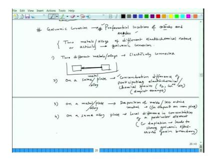
Now, whenever we talk about preferential locations of cathodes and anodes it can happen on the same plate due to concentration effect that is what we have in the understood in the rain droplet example or it could happen some metal deposition. And that metal deposition can happen because for example, if we talk about one example I have cited that is the copper deposit on the steel plate and that copper deposit can lead to a galvanic effect, ok. So, that is also there.
