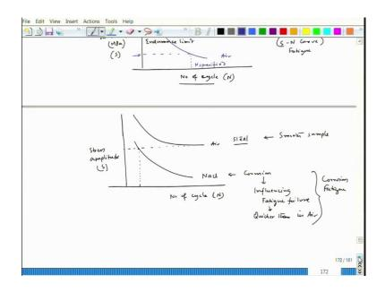
Let us say we have a steel and that is actually exposed to alternate loading you know corrosive solution. Let us say if it is air, it will have its usual endurance limit this is air. But in case of this is steel let us say, but if it is in corrosive, let us say NaCl solution. So, then things will this all those stress amplitude level will go down and it will not have any sort of or kind of plateau region.
