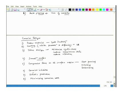
So, there are couple of measures one can take. So, corrosion fatigue. So, 1 is better material and better material means good ductility. Coating, which prevents hydrogen diffusion. In fact, nowadays that petroleum industry where hydrogen assisted cracking is observed those low carbon low alloy pipeline steel.
