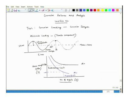
So, the course is corrosion failures and analysis and this is lecture 42 and topic is corrosion cracking. In that we will talk about corrosion fatigue. We know fatigue that if there is alternate loading and there is a tensile component in that alternate loading, the material fails quickly ok.
