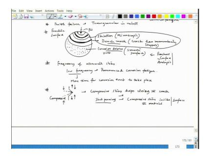
Now, if we talk about fracture surface. If we see this fracture surface let us say there is a pit small pit. So, this is the pit where corrosion fatigue initiates and from that there would be a radiating lines like this and after that this part which will be rough in nature. In most of the cases when we have corrosion fatigue, we will have corrosion debris here debris or
