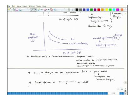
So, in case of notched specimen, this will drop down air and for corrosion for in corrosive solution, this will also in corrosive solution. Now, interesting part is you could see that the gap between these two is actually decreasing and the all the things are dropping down and the level of stress is also dropping down and level of number of cycles at a particular stress amplitude is also dropping.
