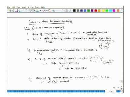
So, let us look at those parts; the protection from corrosion cracking. Now, when we talk about corrosion cracking let us look at SCC or stress corrosion cracking. Now, if we try to see, we have seen that different materials behave differently in different solutions. So, in a particular solution we can choose choice of material. We can choose a material that apparently that does not show a serious stress corrosion susceptibility in that particular solution.
