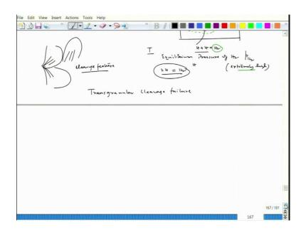
And, the surface looks like kind of radiating kind of surfaces. So, this kind of appearance one can look at without having a specific grain facets. So, this is typical cleavage feature, you can also go to net and then have a look at it what is that the look of cleavage feature.
