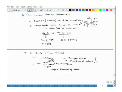
And, the last one what we can you can thought of is basically the atomic surface mobility mechanism. In this case some of the species in this in the corrosive media. So, this is the
