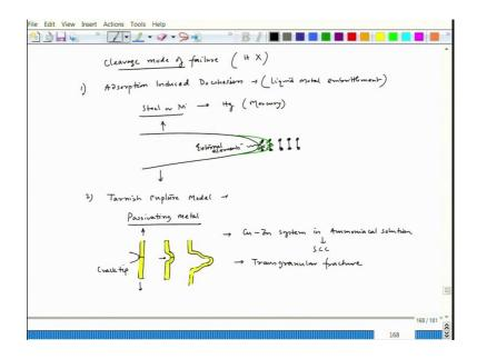
Now, coming to other cleavage mode of failure, so if we talk about cleavage mode of failure so, there where hydrogen is not involved ok. So, the one can think of just like decohesion model, the hydrogen decohesion model, where hydrogen is actually reducing the bond strength or the surface energy. And, if surface energy reduces then fracture stress also reduces as we have seen in case of hydrogen induced decohesion model.
