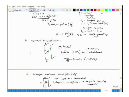
Now, this is the fracture stress this is now when what happens this hydrogen reduces the gamma s. This hydrogen gamma s reduces because of the hydrogen diffusion into the
