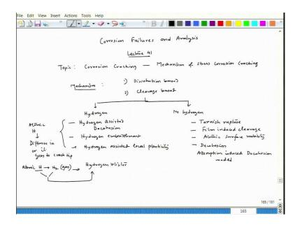
So, the course is corrosion failures and analysis, corrosion cracking and in that we will talk about mechanism of stress corrosion cracking. And, in fact, while doing while understanding mechanism of stress corrosion cracking, we will also talk about hydrogen induced cracking or hydrogen assisted cracking as well as corrosion fatigue.
