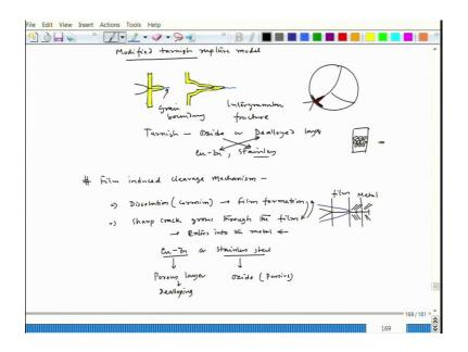
So, in order to address that, so, there is a modified tarnish rupture model ok. So, in that case what happens? This feature what is there in the beginning we have the same operation going on so this is the film ok. And, this film we have a crack that is going in and that crack will lead to a small fracture here in the film. And, then the film will grow into the and let us say there is a grain boundary.
