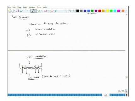
Now there are two modes of fretting attack one is if we try to see the modes fretting corrosion, one is wear oxidation and second is oxidation wear. Now if we try to look at two mechanism, this is wear oxidation if we try to look at two meeting surfaces that meeting surfaces we cannot make it there will be definitely some wavy nature on that meeting surfaces aspirations would be there.
