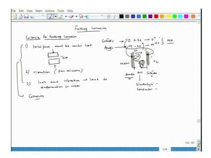
Now let us look at another form of erosion corrosion which is fretting corrosion see if we recall we have discussed in the beginning of erosion corrosion that fretting happens when two meeting surfaces are tight fitted ok and there is a small very small even few microns level of amplitude of vibration so that particularly led to a kind of fretting action between those interfaces.
