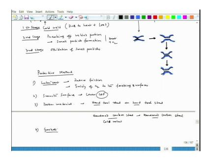
Now third is better material and here it is not about one material both the materials are to be considered because for example, in case of fish plates we have rail material as well as the fish plate itself. So, between that fish plate and the rail we have fretting surface, now better material we have to have a combination of those materials.
