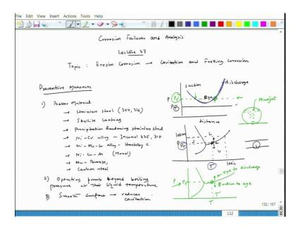
So the course is Corrosion Failures and Analysis and lecture 37 topic we will Erosion Corrosion with the spatial emphasis on cavitation and fretting corrosion. Now if we have we have seen that the cavitation damage happens when bubble collapses on top of a metal surface and that leads to micro jet impact on the metal surface and also the shock waves.
