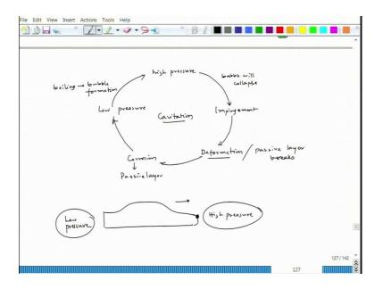
First is low pressure then boiling happens. Boiling leading to bubble formation. Now, if it goes to high pressure, so, then there the operation would be bubble will collapse because vapor will convert to water. So, this bubble collapse will lead to impingement and that impingement will lead to deformation.
