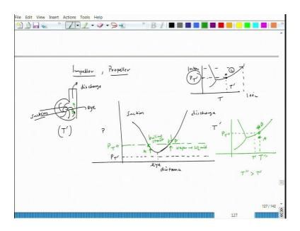
So, there we have cavitation and where we can have those kind of situation? Like impeller, propeller. So, those kind of situations we always experience low pressure at the back of the blade of the impeller, back of the blade of the propeller ok. So, there water can boil.
