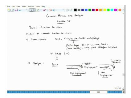
So, let the top, the course is corrosion failures and analysis, lecture 35 and topic Erosion corrosion and in fact, we will start with methods to combat erosion corrosion. Now, when we try to talk about methods, then 1st thing comes better material, hard as well as strongly passivated metals and alloys are good.
