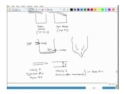
The another design for example, if you have a tank, let us say we have a tank. This is a tank and one way is a pipe is coming, pipe is directed to the center of the tank and in another case, pipe is actually coming and water is coming and hitting the wall of the tank.
