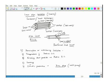
So, these are the design factor. But I would like to consider one small incident that is we call it inlet pipe corrosion. In fact, this corrosion is involving erosion, fine. Now, in that happens in case of condenser or heat exchanger. So, what it is basically? So, now, we have this is a design, we have condenser or heat exchanger. So, this is circular tube fine.
