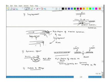
And, if this is my let us say pipe thickness this zone if we draw it in a and zoom it and then see this. So, this is like this ok, now here we have water flow or the fluid flow is going through this and here we have a kind of turbulence, ok. So, this turbulence will have a greater corrosion erosion corrosion here in this portion greater erosion corrosion erosion corrosion.
