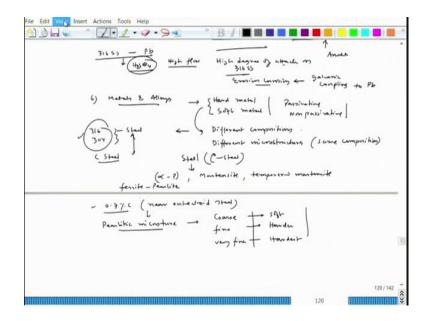
Now, on the metals and alloys, we have talked about hard metal soft metal and then of course, passivating as well as non-passivating kind, fine. When we talk about this hard metal, so, the hard metal and soft metal it can come from different metals different compositions as well as different microstructures in a same composition, fine.
