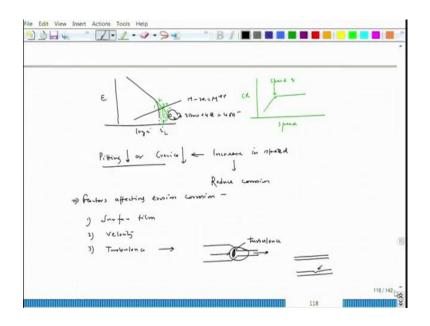
For example, if we recall a mixed potential theory, there if it is if the metal is the metal corrosion is controlled by diffusion mode so, that time this is potential, this is log i which is the plot would be corrosion let us say this is the kind of attack that happens. Let us say this is the metal dissolution part metal minus 2 equal to metal plus 2 the anodic part. So, this is the cathodic part, let us say which is guided by oxygen diffusion.
