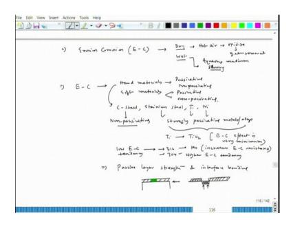
So, the erosion corrosion instead of erosion corrosion I can simply say E-C ok. So, this erosion corrosion can happen in both dry medium or wet medium. So, now, coming to the variation whether we can have it in dry medium; for example, if hot air going hot air is passing through a pipeline. So, then hot air can oxidize the surface and this oxidized surface can get removed. So, the so, this surface can get removed due to the erosion factor and then erosion corrosion or corrosion can take place.
