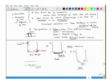
Two different metals, for example, washer and bolt, they could have different compositions, but there could be possibility of metal itself due to design create crevice. One classic example what I showed you last class was basically a ripple rebar. So, ripple rebar is basically like this fine. So, this is the ripple rebar right. So, now, this is the foot of the foot of that particular ripple or rid this called ribbed ok. So, this particular part is creating a tiny crevice.
