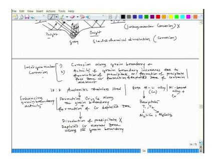
One is of course, corrosion along grain boundary ok, second is this activity of grain boundary increases due to formation of precipitate or formation of precipitate free zone or formation of depleted zone of certain element, fine. So, then only we can call it intergranular attack fine otherwise we do not term them as intergranular corrosion.
