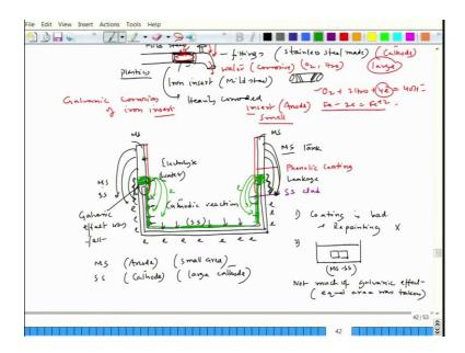
The problem is such that this is a large tank and this tank is made of mild steel MS pipe MS tank, right. Now, after 20 years it was replaced and while replacing people thought that the bottom part because, bottom part is mostly having corrosion related issues, they thought that the let us protect the bottom part.
