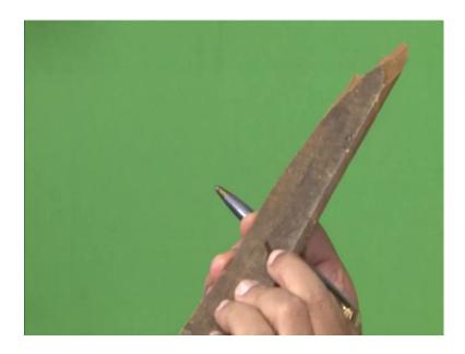
But if you see the inside part it is not for a long duration use, it was maybe couple of months. And then, what happen if you see the screw part inside part the thread of the screw has completely gone, if you see the thread of the screw is completely gone, but at the same time the corrosion that rust deposit is also there, ok.
