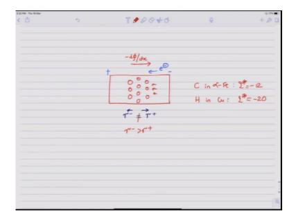
Let us try to look at it. Consider this sample in which I have shown different atomic planes here. In the absence of any electric potential gradient or any external driving force, these atoms are continuously vibrating and their jump frequency in forward or reverse direction are same.  $\gamma^+$  and  $\gamma^-$  are same. Now, consider if there is an electric potential gradient existing from left to right as shown here and the electrons are flowing from right to left.
