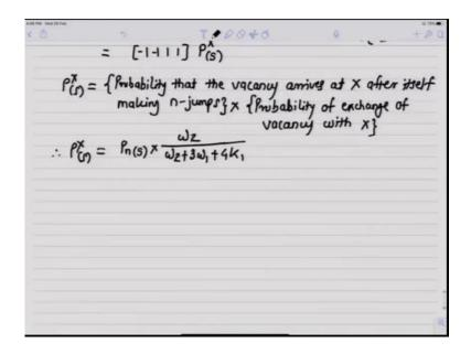
Now, let us recall this probability that the vacancy arrives at X after itself making n jumps as  $P_{n(S)}$  and the probability of exchange of vacancy with X is  $\omega_2$  divided by total number of jumps per second that the vacancy can make. So:
