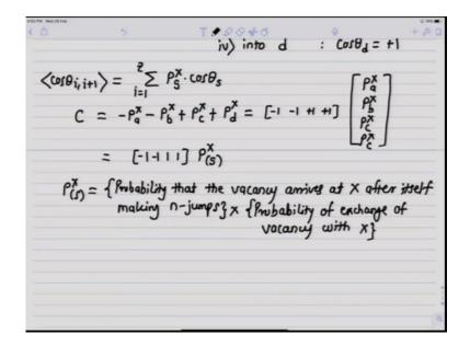
$P_S^X$  is here is the probability that the 2nd jump of atom X is into the site S.  $\cos \theta_S$  is the cosine of the angle between the 2nd jump vector and the 1st jump vector which was aX. Now there are 1a type of site, 3b types, 3c types and 1d type.
