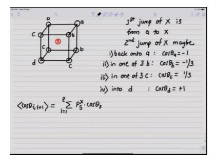
Let us redraw this BCC unit cell again and now in this cell I have shown the tagged atom at X at the body centre of this cube. Suppose the 1st jump of the atom X is from this site a to X. the 1st jump of tagged atom X is from a to X. The second jump of X maybe on one of the eight sites and those eight sites, the nearest neighbour of X can be divided into sites of the types a, b, c or d. a is from where the X has just jumped during the 1st jump. So:
