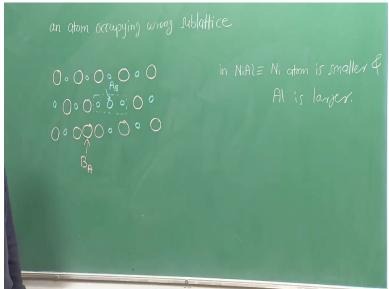
Next type of defect is called an Antisite. As the name suggests, it is an atom, occupying site on a wrong sub lattice. B atom occupying an A sub lattice site or an A atom occupying a B sub lattice site is called an antisite. Here you can see, this is an A atom which is wrongly placed on a B sub lattice. This is an antisite of A on B, we denote it as  $A_B$ . If we have a B atom occupying an A sub lattice, like here this is called as antisite of B on A, it is denoted as  $B_A$ .
