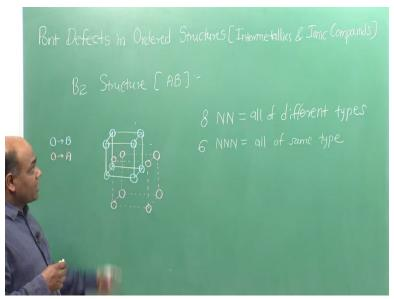
The first one of it is called a  $B_2$  structure and the intermetallics or compounds with the stoichiometry of the form AB exhibit this type of crystal structure.  $B_2$  structure basically can be looked at as an interpenetration of two simple cubic sub lattices. One for type A atoms and the other for type B atoms. If we draw a single cubic cell, it resembles a BCC unit cell with all the corner sites occupied by 1 type of atom and the body center occupied by the other type of atom.
