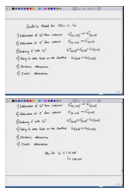
He considered the monovacancy formation in copper and he split the process in 6 different steps. In a metal, metal ions are held together at their regular lattice positions by the cloud of electrons. The first step he considered was sublimation of one copper ion from the interior. He denoted this as  $Cu^+$  from solid and the interior of the solid to  $Cu^+$  in gas state to infinity:
