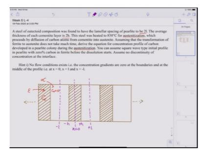
The problem is a steel of eutectoid composition was found to have the lamellar spacing of pearlite to be 2l. So, the period here is 2l, the average thickness of each cementite layer is
