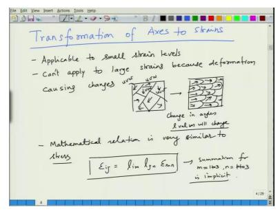
Now what we are going to do is that, we are going to do transformation of, we are going to apply the transformation of axes to strains. We saw the transformation of axes to stress. Now we will look at the transformation axes to strains. So now this is applicable only to smaller strains. We cannot apply to large strains because of deformation causing changes.
