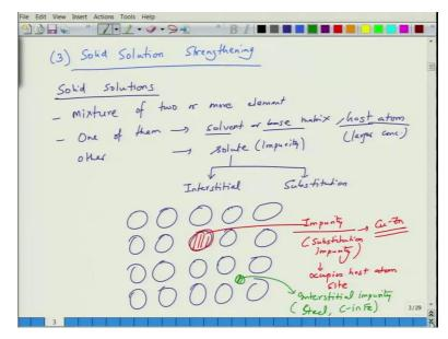
Now, the third method of strengthening is called as Solid Solution Strengthening. So, basically here what we do is that. So, we know what solid solutions are? Solid solutions are solid solutions are mixture of two or more elements and generally one would be the base, one would be in larger concentration than the other. So, basically you can say one of them is solvent or base, it is not liquid form.
