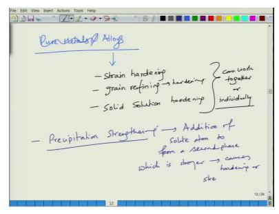
However, let me just, so if you do not form second phases. So, let us say, so pure metals and so let us say, we talk about alloys. In alloys, we can do strain hardening, we can do grain refining and we can do solid solution hardening and all these three mechanisms can work together or you can make them work. So, can work together or individually.
