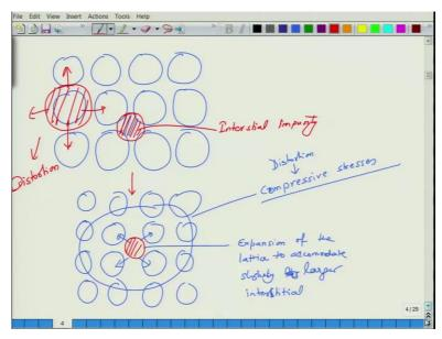
Now, what the, what this does is basically when you have let us say a structure like this. So, these are host atoms. So, if I put a interstitial impurity which is slightly bigger than the size of the interstisis. So, the my interstitial impurity is like this, it is slightly bigger. So, what it is going to do is that, it is going to displace these host atom.
