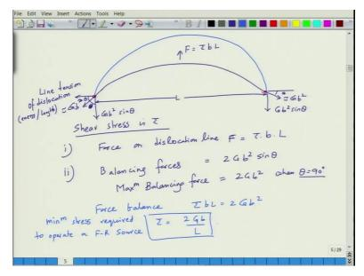
So, you have a loop like this and these are pinning sites and the distance between these is given as L. So, the force on the, so the distance is L and these are the pinning sites. So, the force from the dislocation when shear stress tau is applied. So, shear stress is shear stress is tau.
