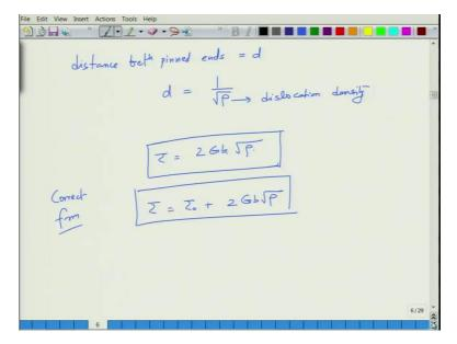
So, basically what we have done in this lecture is, we have looked at the sort of semi quantitative analysis of stress that is required to operate a Frank Read source this we have done by doing a simple force balance.
