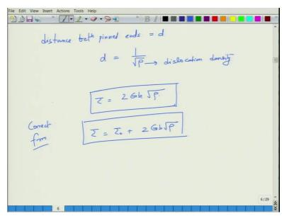
And says that distance between pinned ends is d and this d is related to dislocation density as 1 over square root of rho. So, this is rho is dislocation density, so because dislocation density the unit is number of dislocation per meter square, so it goes as 1 over. So, basically rho as 1 over d square or you can say that d goes 1 over square root of rho. So, if you write this stress then it becomes 2 Gb into square root of rho.
