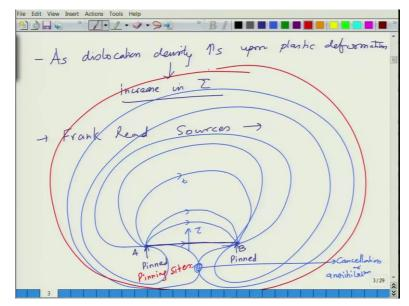
So, basically what we see is that as dislocation density increases upon plastic deformation this also leads to increase in stress that is required to move the dislocation so (())(3:31) plastic deformation. So, basically that is what is strain hardening. So, the reason for that we will see later on but first of all we saw that you have Frank Read sources leading to dislocation generation and what we saw that you know you have dislocation like A B.
