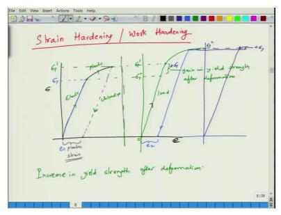
So and we see this experimentally because when you do stress strain curve wherever you stop the deformation and when you again restart deformation. So, this is restarting the deformation again when you restart the deformation you increase the yield strength by little bit corresponding to how much you where you were on the stress strain curve at the end of previous deformation.
