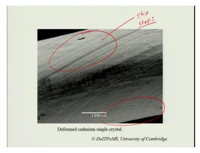
So, when you start deforming it, this is a deformed cadmium single crystal when you start deforming it, then you see you can form these step on the surface. So, these are basically, so you can see the steps here on the surface you can see the steps here. So, these are basically, you can say the slip steps, which have formed because of slip of atoms against each other in successive planes in the slip plane of course the slip has to occur in the slip plane.
