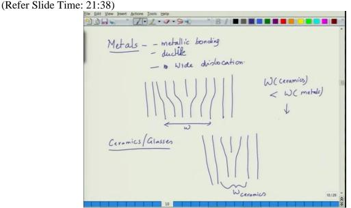
So, basically in metals, which show metallic bonding and are ductile, they show wider wide dislocations. So, schematically speaking you can say in a, in a meatal the scenario would be. So,
