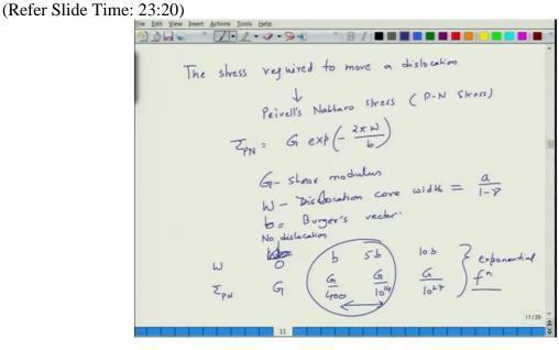
But the stress which is called as Peirells Nabharo stress or P.N stress and this is given as tau P N G into exponential of minus of 2 pi W divided by b. So, here G is you know the shear modulus and W is the dislocation let us say core width and b is the Burgers vector and W is also given as W is approximated as a divided by 1 minus nu.
