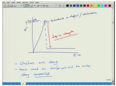
So, this is a stress-strain test on Whisker and when you apply the stress basically, you go to a value of nearly. So, let us say this is stress-strain curve on Whisker. So, you reach a strength of order of let us say 700 MPa which is close to 1 GPa very high strength and then when you reach very high strength you are able to reach some bonds and at this point you introduce a defect or dislocation and this is where there is a sudden, drop in strength.
