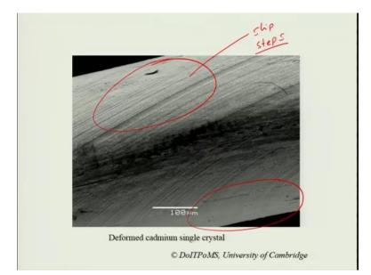
So, you can see this, this is what is happening, if you look at it microscopically at a further high. So, this magnification you can see that here its scale bar is 100 micron. Now if you increase the scale part, if you increase the magnification reducing the scale bar to 5 micron, you can see that these are microscopic steps that you form on the surface of the sample.
