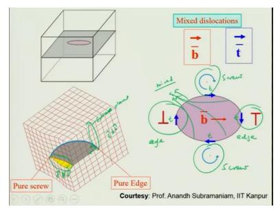
In reality what happens is that, we have a dislocation, which could be something like this in a form of loop or it could be in this in which on one side if you look at the crystal it looks like a screw dislocation. So, this is the screw component, because the burgers vector, parallel to the slip line. But here if you look at this part of the crystal, this is the edge part.
