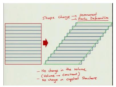
So this how it is going to look like. So a perfect crystal when deformed by motion of dislocation in the successive plane, it leads to creation of these steps and you can see that it creates a deformation, what happens basically is there is no change in the volume. Volume remains constant. So, the constancy of volume has to be followed, there is no change in crystal structure which means the crystal structure of the material does not change.
