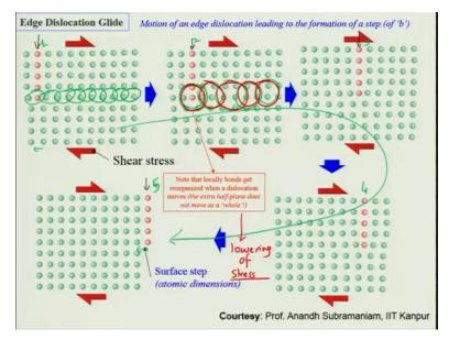
So, how does this dislocation move basically the motion of a dislocation leading to the formation of step. So, let us say you have this extra row of atoms here, you go from here to here. When you apply shear stress, so this extra row moves to the next one. So, which means this row goes in this fashion, this will come forward.
