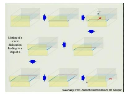
Similarly, screw dislocation if you have a screw dislocation like this, this is a prefect crystal this is the screw dislocation and as you keep applying the stress in this direction, this dislocation line moves in this direction the step gets created across the whole crystal when you come here finally, you have this extra step b.
