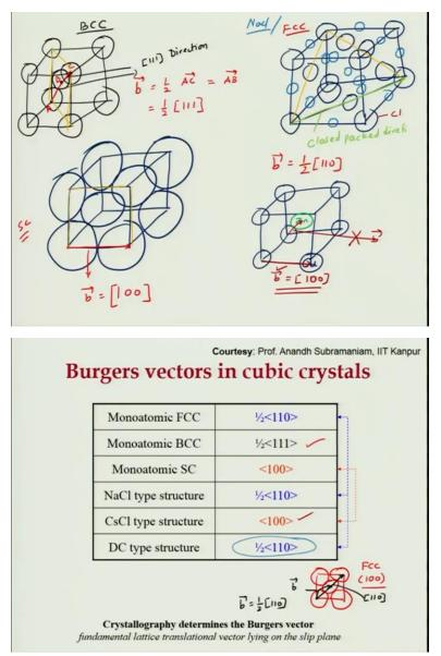
In the next one, so this is for the example BCC and you have one extra atom in the center. So, assuming that all of them touch each other, the closed packed direction is the direction which is this direction. So, closed packed direction touches this, this, this and this. So this is your, you can say 1 1 1 direction for BCC.
