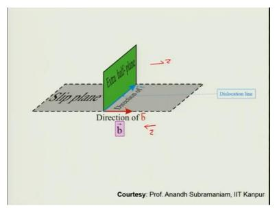
And the plane one which this extra row of, extra plane of atoms moved can be visualized in this fashion. So, you have this slip plane, in the slip plane this extra half line will move either to the left, either to left to or the right depending upon the stress. But and the line adjoining this extra half plane is slip plane is the slip line.
