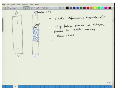
So, essentially you can see that you have a wire like this and as you start deforming, the wire surface will show these, it will get longer and it will show these kind of steps on the surface. So, all tough you are applying the stress along this axis, the movement of planes is happening in this direction. So, which means, there is a shear component that is acting. So, plastic deformation as we are saying happens by slip.
