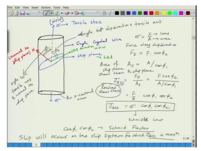
So, this is, this is what you have, you have a material whose schematic, let say a wire. A wire with across certain, certain cross section and this wire is subjected to a tensile stress. So, this is sigma, this is sigma. So, this is tensile stress that is applied to the wire. In this wire, it has certain orientation. Let say, u v w. Let us say this is a single crystal wire. So, this is signe crystal wire, let say it has a slip plane which is oriented like this.
