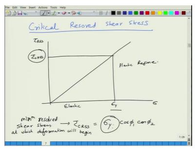
And what you can see is that, this resolved shear stress gives rise to a concept of what we called as Critical Resolved Shear Stress and basically what it means is that, if you plot tau RSS as a function of sigma and sigma keeps increasing.
