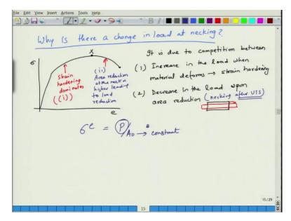
But first the question is, why is there a change in the load at necking? At necking we see that the load changes like this. So, this is the point let us say x sigma e. So, there are two things which happen, it is due to competition between first, you have strain hardening that is happening, so increase in load. There are two things which are happening when material deforms, increase in the load when material deforms due to strain hardening.
