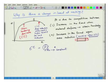
And it is the necking, which is important turning point in the deformation. And that is why generally from engineering perspective we do not deform the sample beyond ultimate tensile strength. And so, we will further look at the behaviour, this tensile behaviour and tensile properties and phenomena of strain hardening and other things in the, and the phenomena of plastic deformation at the microscopic scale in the next few lectures. Thank you very much.
