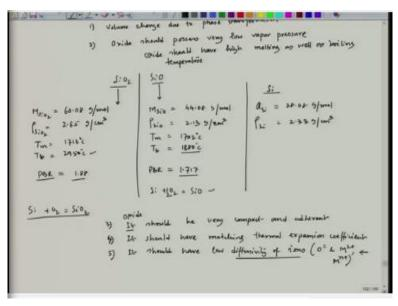
So there are other factors like for a oxide to be protective it should be very compact and adherent, fourth it should have matching expansion coefficient or I would say thermal expansion coefficient, then it means oxide, so it should have low diffusivity of ions and here I am considering O2- and metal 2 + or I can even consider metal n + for example in case of aluminum it will be Al3 + in case of chromium it is Cr3 + whereas in case of iron it could be either Fe2 + or Fe3 +.
