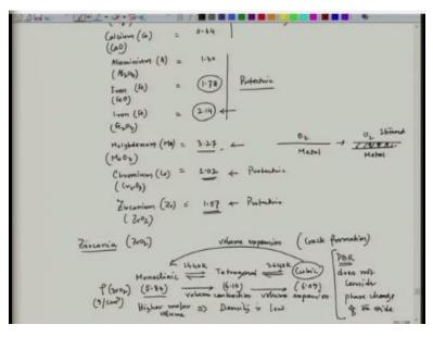
Now you can calculate for other cases some of the metals where PBR ratio is less than 1 let me note it down. For example, if you take magnesium, so that time if I try to put down all those values magnesium is 0.81 and that time oxide is MgO. Then calcium, so that time oxide is calcium oxide, it will be 0.64. Of course we have seen aluminum and oxide is Al2O3 PBR ratio is 1.3.
