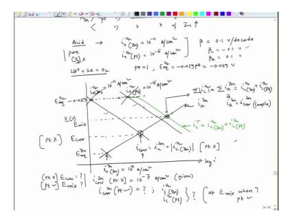
But many times we can have a situation for example, we can have a couple between this particular galvanic coupling where both have same area. So this is extremely important. Will feel it around that if the area of the this galvanic area of the individual component of that galvanic couple are different, the corrosion rate of the zinc of zinc or the active component will change. We will see that if the area of the Platinum.
