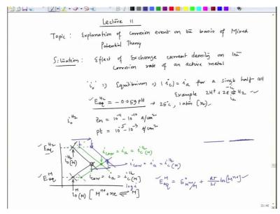
Let's start lecture 11 and topic we will continue explanation of corrosion event on the basis of mixed potential. Our theory in the last lecture we thought that we will be able to complete two situations. One was effect of when a electrochemical process that means corrosion of zinc is taking place in HCl rather impure HCl with dissolved oxygen. So, that case we can have 3 catalytic reaction and 1 anodic reaction.
