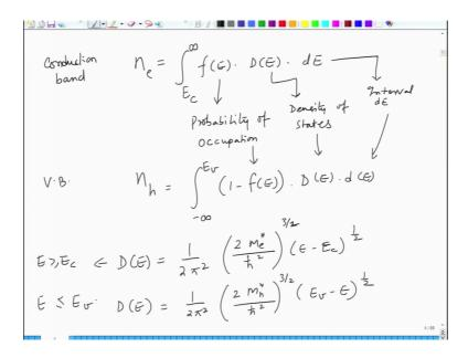
So, the way these carrier concentrations are come about so, the carrier concentrations are basically calculated as so, from E g to in E c to infinity sorry next. So, this is E c to infinity for conduction band. So, this is for conduction band so, this would be  $f \in D \in D$  into  $d \in E$ .
