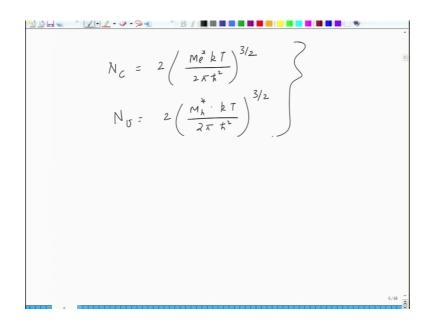
So, this N c N v is basically N c N v is N c is 2 into me star k T divided by 2 pi h cross square to the power 3 by 2 and N v is equal to 2 m h star k T divided by 2 pi h cross square to the power 3 by 2, these are the expressions for N c and N v which we did not look at last time.
