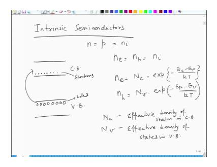
So, moving forward on this discussion intrinsic semiconductors are the ones for which n is equal to p and this is mainly those semiconductor which are where carrier generation is because of thermal excitation.
