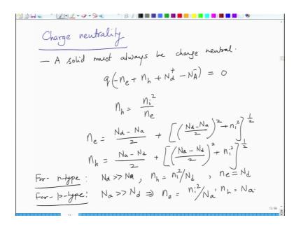
So, which means no matter what happens is that a solid must always be be charged neutral which means that for a given semiconductor q into n e so, minus n e is the negative charge plus holes n h plus N d plus which is the donor atoms minus the acceptor atoms which are negatively charged minus N A minus that overall charge must be equal to 0 and we know that n h is equal to n i square divided by n e.
