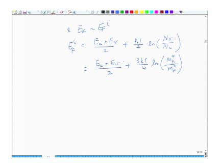
If that is true then we can get the expression for and if E F is defined as E F i, then we can write an expression for E F i; E F i is equal to E c plus E v divided by 2 plus k T by 2 into ln N v by N c and this will turn out to E c plus E v divided by 2 plus 3 k T by 4 ln of m h star divided by m e star effective mass of hole electron.
