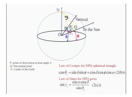
Now, you can represent the whole thing in a different way in this kind of with respect to earth being is a sphere, and sun being somewhere around it; so, which is sort of a legitimate design. And again using the equal law of the cosine, you can determine cos theta z will be equal to sin theta sin phi plus cos theta cos phi cos omega.
