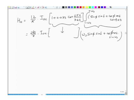
So, how do you work out? Now, H naught this H naught is the monthly the average of extra terrestrial radiation that would fall on the on a horizontal surface. H naught is given by this equation, 12 divided by phi into I s c which is the solar constant into 1 plus 0.033 cos of 2 pi n divided by 365, and then you integrate it over whole day.
