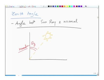
Next angle that we determine is zenith angle. Zenith angle is the angle between sunray and a normal. So, essentially this is the normal, this is the horizontal, this is the sun and this is a sunbeam, the angle here is called as theta z, this is normal.
