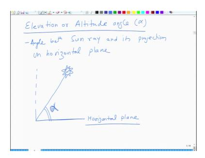
So, the first angle that we define is called as elevation angle or altitude angle, which is called an alpha. This angle is defined as the angle between some ray and its projection on horizontal plane. So, let us say this is the vertical this is the horizontal plane, this is sun, this is the sunbeam that is coming. So, this is the value which is called as elevation. So, you can say this is alpha, right. And then you calculate so this is let us say horizontal plane (Refer Time: 15:36).
