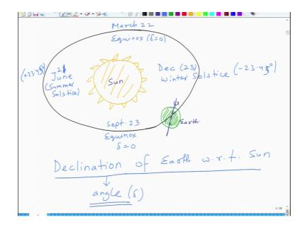
And let me just correct the values this is 45, ok. So, the first angle that we have worked out is delta which is a declination angle is 23.45 degrees multiplied by sine of 360 divided by 365 into n minus 81. So, naturally you can see the value changes form plus minus 23.45 to plus 23.45 degrees as a function of day of the year.
