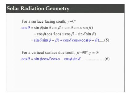
So, for example, to simplify the matters, if you have a vertical surface which means beta is equal to 90 degree, then cos theta can be simplified by combining the above 3 equations as sine phi cos delta cos gamma cos omega minus cos phi sine delta cos gamma sine beta plus cos delta sine gamma sine omega that is the first relation that gets modified for a vertical surface.
