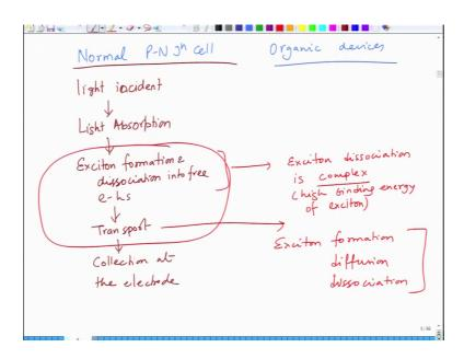
So, we know that in a solar cell what happens is that we have you know light comes on to the solar cell; then it you absorb the light. So, you know in a normal solar cell; so first step is you have light incident, then light absorption, after light absorption you have excitons formation and dissociation into free electron and holes after this we have separation of charge.
