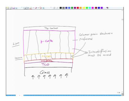
So, we have glass substrate. So, this is glass transparent glass the light comes from this side, and then we have TCO. So, you can have a TCO here TCO means Transparent
