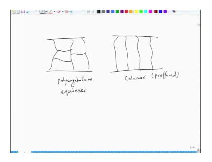
Columnar grains are good, because see you can have a in a device, you can have a grain structure like this; like this or you can have a grain structure which is like this. So, this is you can say a polycrystalline equiaxed grain structure, and in this case you have so this is a preferred grain structure, because it prevents recombination sideways.
