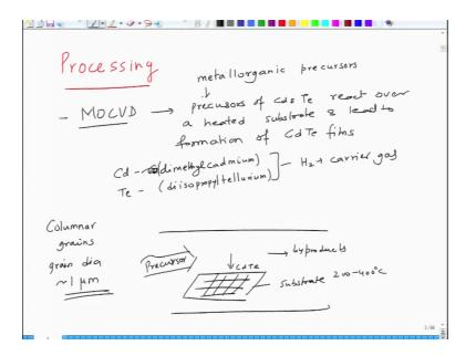
So, as we said about processing. So, not only you can process CdTe by sputtering evaporation galleria reaction, you can also process this by MOCVD kind of process, where in you know the precursors of Cd and Te react over a heated substrate and lead to formation of cadmium telluride film, and these precursors are basically metallorganic precursors.
