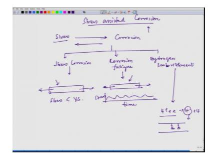
And finally we have stress assisted corrosion. In case of stress assisted corrosion as the name suggest again. So, we have corrosion and then stress is also helping or it can be other way around, stress should be there corrosion would also aggravate the attack. Now, stress associate corrosion. They can be divide into three parts: one is Stress Corrosion, another one is Corrosion Fatigue and then, high we have Hydrogen Embrittlement.
