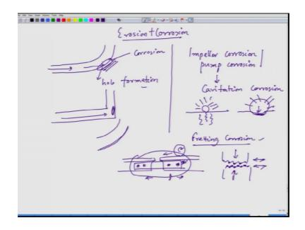
So, let us go to the another form of corrosion which is erosion corrosion. In case of erosion corrosion, as the name suggest that there would be a flow which we will involve wire of this material and plus corrosion so; that means, erosion plus corrosion. So, like a kind of pipeline, where we are flowing water and that water if it contains suspended particles.
