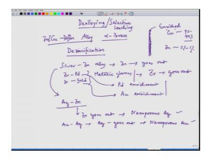
So, we are left with four other forms one is dealloying. Dealloying a kind of corrosion form, where one of the elements in an alloy preferentially dissolves. For example, if we consider copper zinc alloy, if we consider 70 percent copper and 30 percent zinc which is called alpha brass, there we do experience dealloying where zinc which is very active component when copper and zinc are together.
