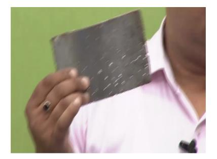
Now, as we have mentioning that the pit can be so dangerous. I just would like to give you one example. This is the plate. Let us look at this plate and this plate the material is 304 stainless steel and when we see this 304 stainless steel, we have a kind of idea that stainless steel means it should be stainless that means, the corrosion would be minimized.
