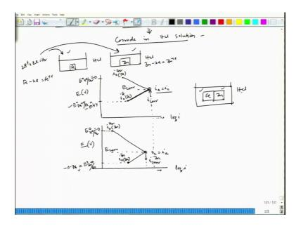
I am just drawing one after another and this is one below another. So, log i this is also log i this is E this is E volt, volt let say this is E 0, hydrogen equal to 0 and let say this is E 0 zinc plus plus zinc which is equal to 0.76 volt.
