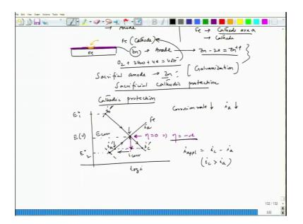
Exactly this similar situation happens when we have iron phase, this is iron and on top of it if I put a zinc layer zinc layer, this is the red colour is the zinc layer. So, until and unless zinc is covering iron surface we have one single reaction which is zinc dissolution. But the effect of zinc on the iron corrosion will take place whenever there is a opening. Let us say this is the opening part, now this opening region is basically iron this is iron and rest of this case is zinc.
