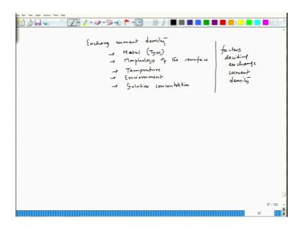
So, now, there are other factors on which this exchange current density depends. It depends on as we have said metals type, morphology of the surface, then we have temperature environment. Why environment because sometimes we have a situation like in one place we have higher salt content or in other place we have less salt content. Then
