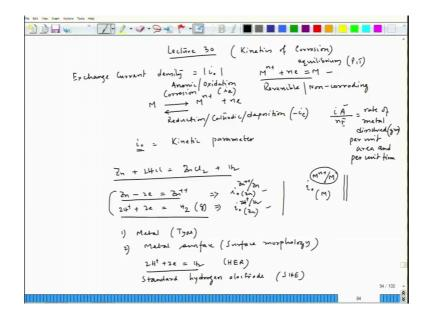
And will continue our discussion on kinetics of corrosion and we have been discussing on current density and we saw the concept of i 0 also which is called exchange current density, which appears when for a particular redox reaction. For this particular redox reaction when it reaches equilibrium.
