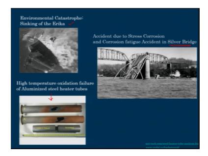
Now, if I see some of the pictures for example, this picture this is a kind of oil vessel Erika, this failed due to corrosion. This is a major reason that this failed this broke into half actually. Now this is the kind of failure I was talking about this is a silver bridge silver bridge failure, and I think it is it happen in 1967. And again if you come to see this part this particular situation, this is high temperature oxidation failure of aluminium steel heater tubes.
