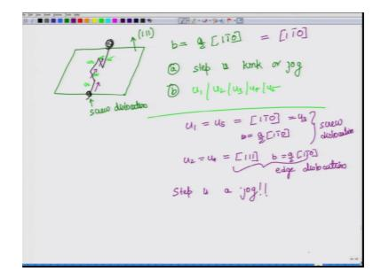
So, in this particular example we used edge dislocation. Next we will try to do the same thing with a screw dislocation. So, here the screw dislocation is given to you here this is the screw dislocation and this is coming out of plane this step then there is a section parallel to this, then again coming back. And here and this is a hole screw dislocation and it is given that this is 1 1 1 plane and the burger vector for this is given as a by 2 1 1 0.
