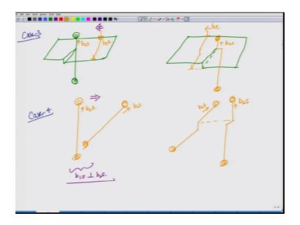
Now here we will have one screw dislocation involved, we will not be able to show the plane for the screw dislocation for the slip plane, but we will try to show the plane for the edge dislocation. So, let us say the screw dislocation is like this. So, this is the plane and
