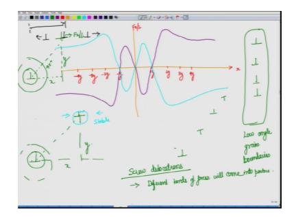
So, what we will do is well on the y axis well have the F x by L. So, on the y axis we have f x by l, but on the x axis what we will do is we will keep x in terms of y meaning it is. But we will plot it in terms of how many y because we have seen it differ even if you remember from the stress field, it changes at 45 degrees. And therefore, it is much more easier and more meaningful to understand with respect to y. So, we will say x in terms of y 1 y 2 y 3 y 4 y and so on.
