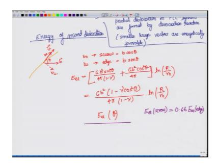
So, how do we find the energy and we showed that you can dissociate or you can find resolve b into edge and screw components; so, the using that we will be able to find the energy of a mix dislocation. So, using the same plot; so, our topic here right now is Energy of mix dislocations. So, let us say the burger vector is like this, which is at an angle theta. And therefore, you have b which is perpendicular to the line vector, which is
