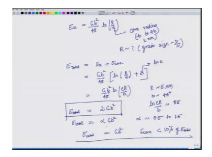
And this is total energy, we also have relation for just the elastic component. In the elastic component, you add a core component energy, core energy where the linear elasticity does not hold and usually this E core is less than 10 percent of the energy ok.
